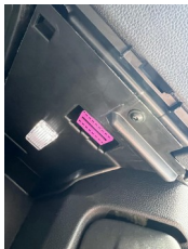
OBD-II port, usually in driver's footwell
