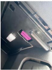
OBD-II port, usually in driver's footwell
